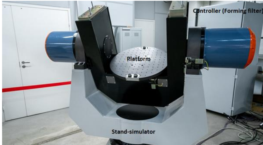
Figure 1. Standard design of an aircraft flight simulator
